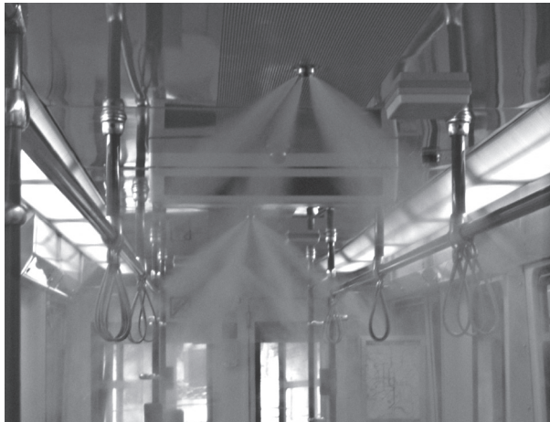
Fig. 2. High pressure water mist fire fighting systems are far the most effective and diffused technology for protection of passenger areas. Here a Fogtec application in a metro train
