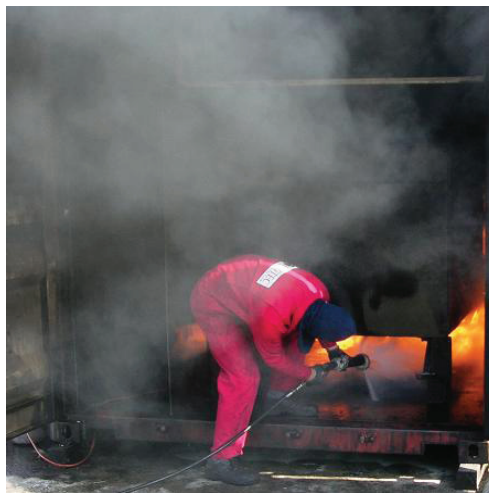
Fig. 11. Extinguishment of a fuel pool fire by high pressure water mist, during FOGTEC full scale fire tests in a mock-up of a locomotive engine room
