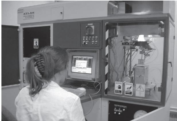
Fig. 4. Tests on cone calorimeter according to ISO 5660-1
