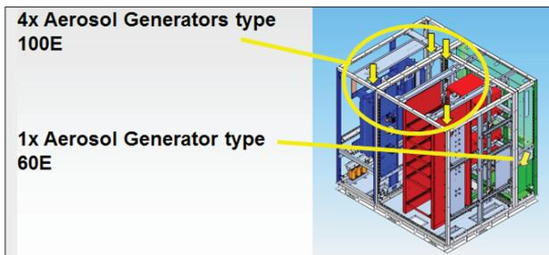
Fig. 5. Example of the position of aerosol generators
