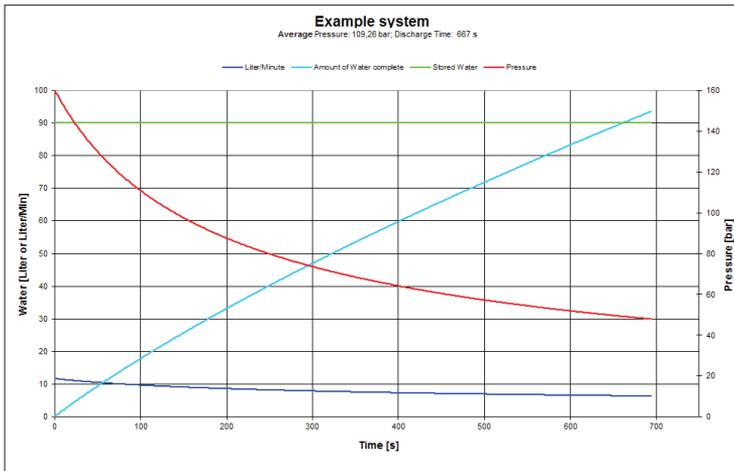
Fig. 8. Calculation of stored water quantity for the passenger areas
