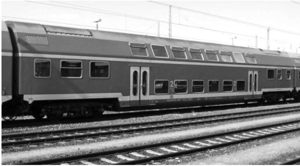
Fig. 2. Coach used for the example is a traditional UIC double-deck coach
