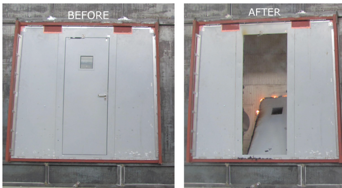
Fig. 7. Example of integrity failure
