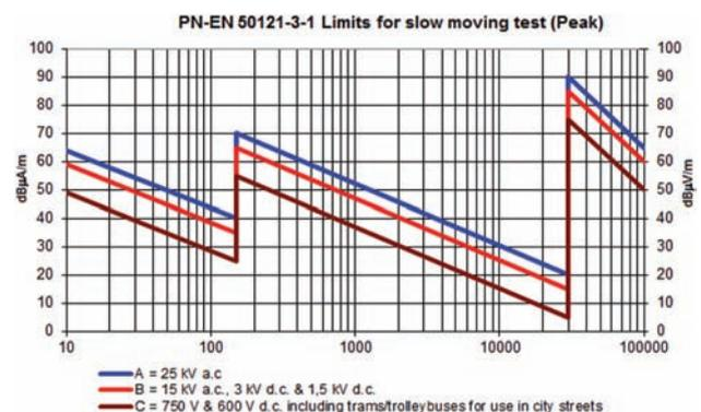
Fig. 3. Permissible levels of radiated disturbance emission for railway rolling stock during the drive [The author's own figure]
