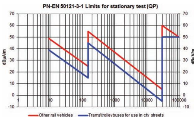
Fig. 2. Permissible levels of radiated disturbance emission for railway rolling stock during the stop [The author's own figure]
