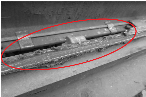
Fig. 3. Damage to switch rails in the form of spallings of material a) and b) [photo. M. Czarnecki]
