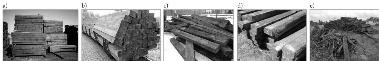
Fig. 3. View of impregnated (a, b) and depleted (c, d, e) wooden sleepers (switch sleepers) removed from railway lines [3]
