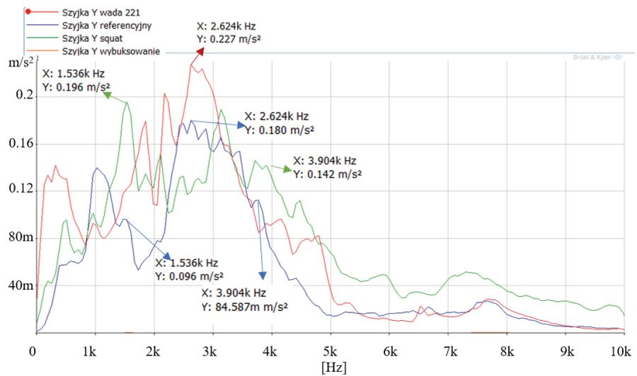
Fig. 6. The patterns of the RMS values of acceleration as a function of frequency for axis Y of the three-axis sensor on line no. 213 [authors' own work]
