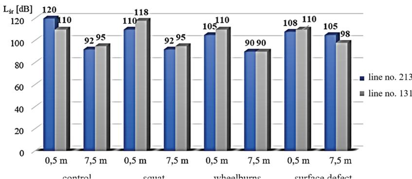
Fig. 5. Average noise level values recorded on lines no. 213 and 131 for different defects at two measurement points – 0.5 m and 7.5 m [authors' own work]
