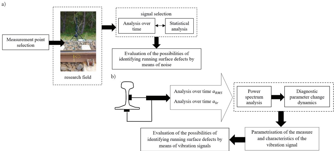
Fig. 4. Procedures of the analysis of vibroacoustic signals in the process of identifying running surface damage: a) acoustic analysis, b) vibration analysis: [authors' own work]
