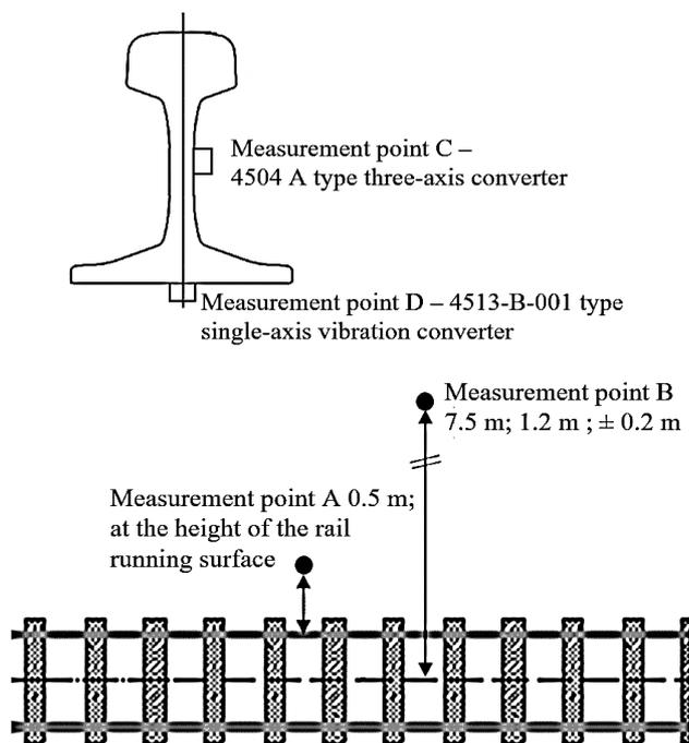
Fig. 3. Arrangement of vibration and noise measurement points [authors' own work]
