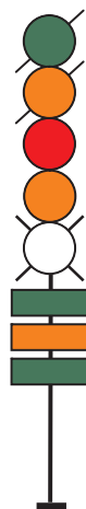
Fig. 2. Three block light semaphore for signaling six travel speed levels [own elaboration]
