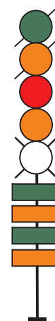
Fig. 4. Three block light semaphore for indicating seven travel speed levels [own elaboration]
