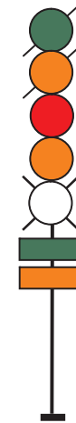
Fig. 3. Three block light semaphore for indicating five travel speed levels [own elaboration]
