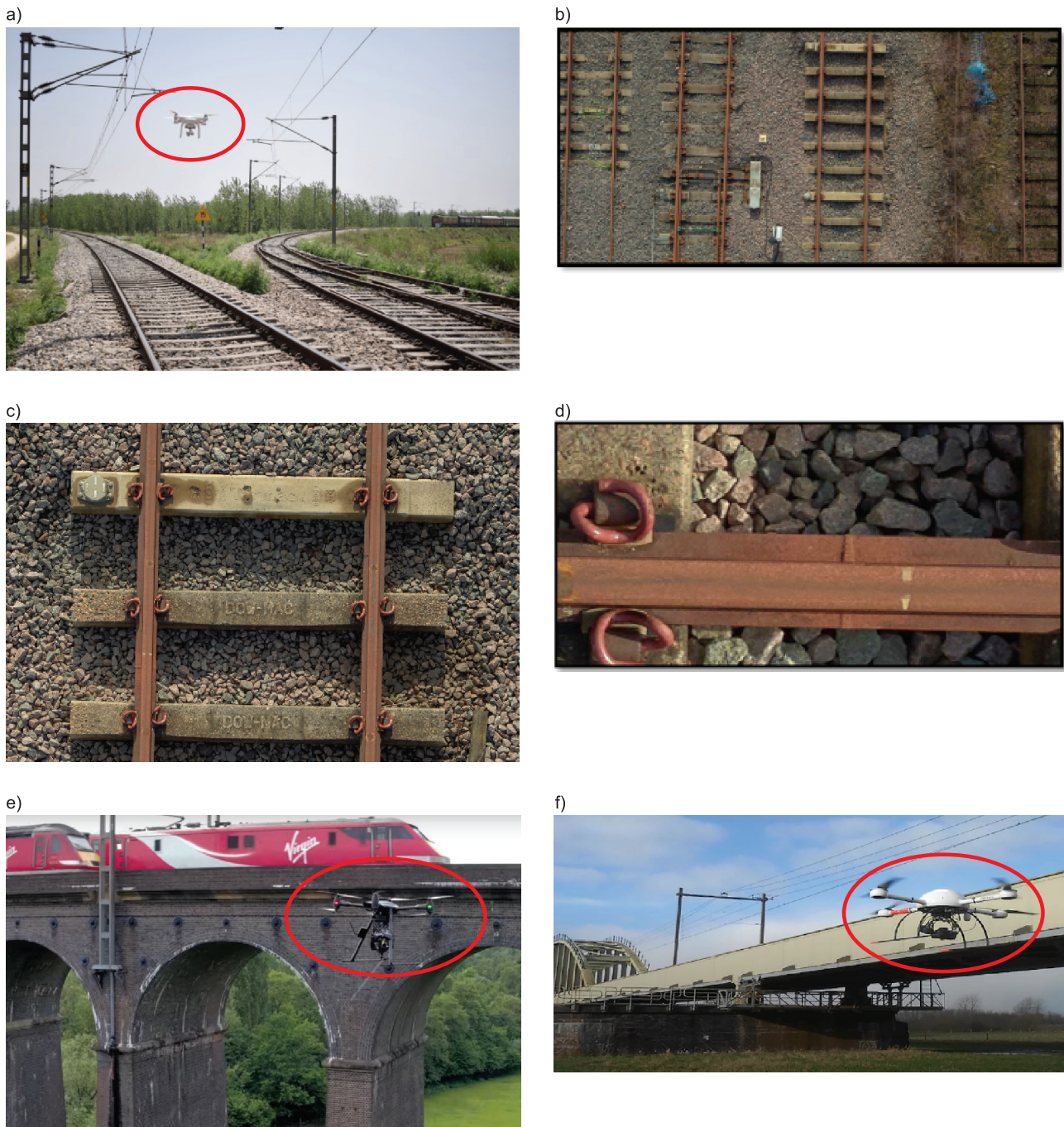
Fig. 2. Inspection of railway infrastructure with a UAV: a) track inspection [13], b) a general view of a track from a height of 25 m [7], c) an approximation of a track section – sleeper designations visible [7], d) a view of a rail with elastic fixations – weld visible [7], e) inspecting the condition of the concrete structure of a railway viaduct [7], f) testing the corrosion of the steel structure of a railway bridge [27]
