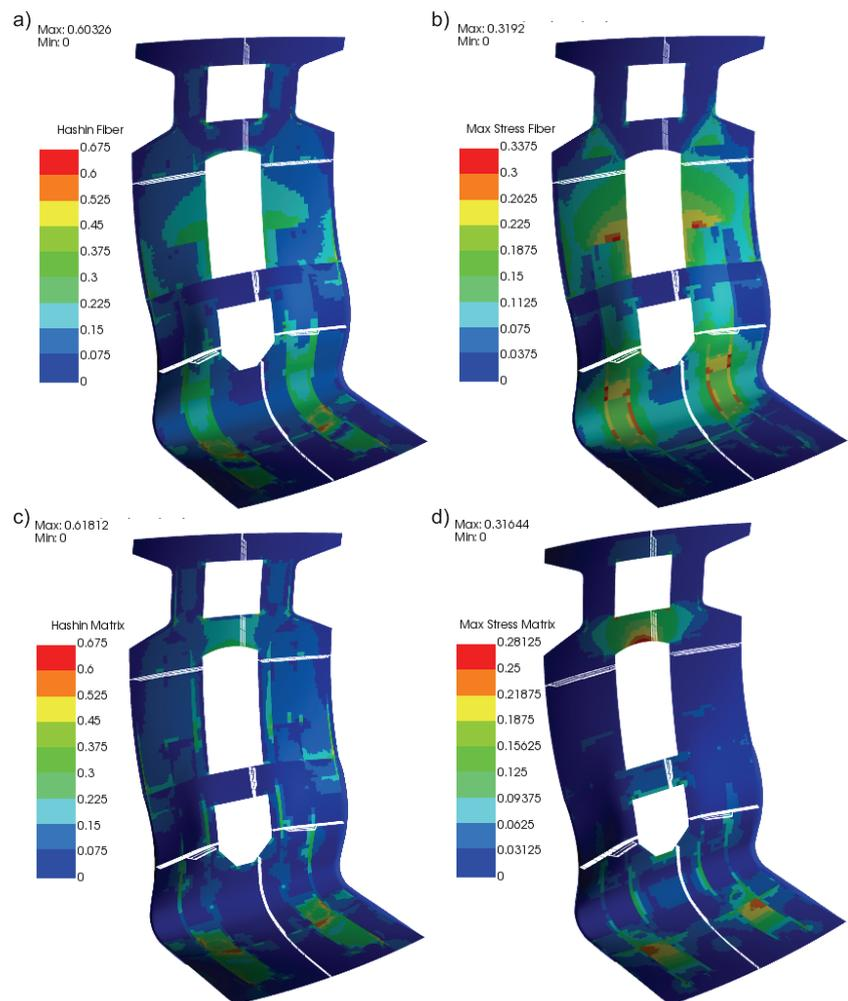
Fig. 13. Distribution of the  $R_i$  failure index for the composite shell model for two selected orthotropic directions 1 and 2 and for two strength criteria: a and c) the Hashin criterion, b and d) the maximum stress criterion [authors' own work]
