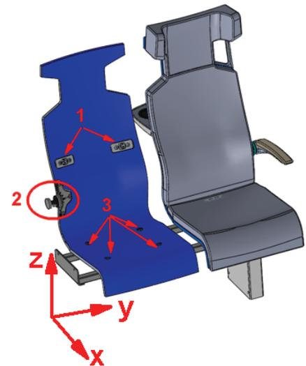
Fig. 8. Attachment products of the equipment fixed to the seat's shell: 1) table, 2) armrest, 3) visible points of fixing to the train car's structure [authors' own work]
