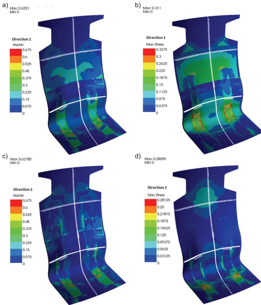
Fig. 11. Distribution of the  $R_i$  failure index for the composite shell model for two selected orthotropic directions 1 and 2 and for two strength criteria: a and c) the Hashin criterion, b) and d) the maximum stress criterion [authors' own work]
