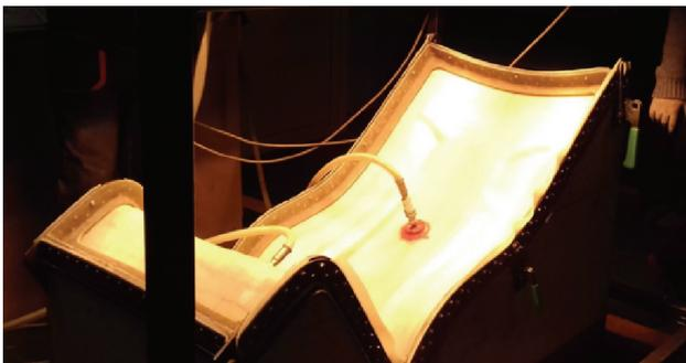
Fig. 3. The stand design for hot vacuum lamination of train seat composite shells [photos by: authors]
