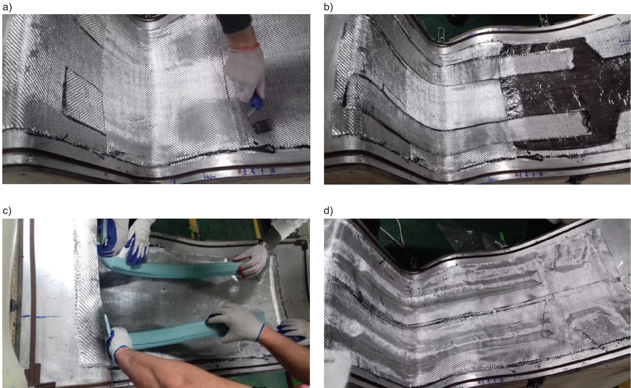
Fig. 2. Examples of stages of laying composite pre-pregs in a mould; a) external layers and layers within the lumbar zone b) polyurethane foam in the headrest zone (black colour) and the first layers forming ribs, c) polyurethane inserts shaping the rib, d) surface layers – end of the laying process [photos by: authors]
