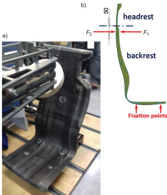
Fig. 5. Seat shell validation model: a) the shell mounted on the test stand and force application punch, b) boundary condition [authors' own work]
