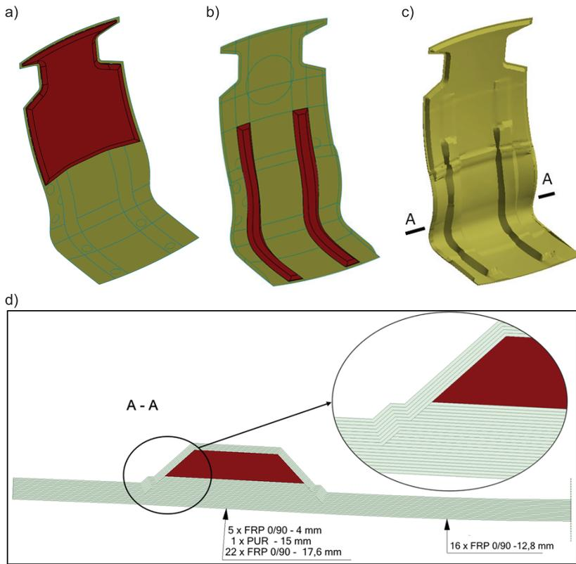
Fig. 7. The structure of the support shell of a train seat: a) PU foam layer in the upper zone of the backrest, b) PU foam inserts shaping the ribs, c) the final geometry of the model, d) 1/2 of the cross section of the lumbar zone with the arrangement of the layers [authors' own work]
