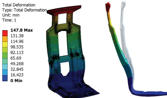
Fig. 12. Total displacements of the shell model [authors' own work]
