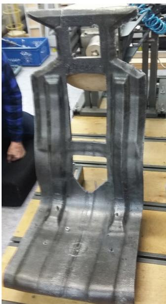
Fig. 6. A train seat composite support shell with holes cut through [photo by: authors]
