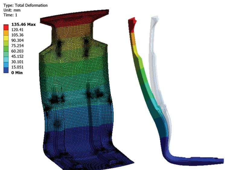
Fig. 10. Total displacements of the shell model [authors' own work]
