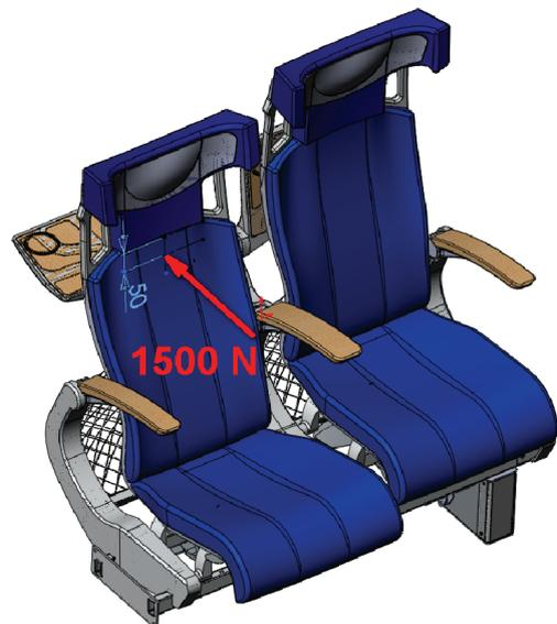
Fig. 4. Point of force application (50 mm below the upper edge of backrest) during strength test
