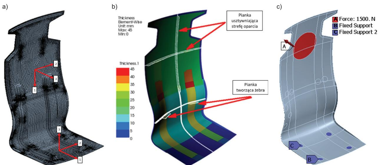
Fig. 9. A numerical model of the train seat's support shell: a) a finite element mesh with marked orthotropic directions of composite layers, b) a thickness distribution chart with colour markings, c) boundary conditions [authors' own work]
