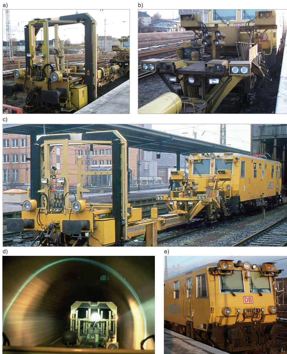
Fig. 8. LIMEZ II measuring set: a) screen frame of the measuring wagon [photo: Thomas Linberg], b) equipment of the measuring wagon frame [photo: Thomas Linberg], c) general view of the LIMEZ II measuring set [8], d) tunnel measurement [14], e) front of the drive unit of the LIMEZ II measuring assembly [photo: Thomas Linberg]
