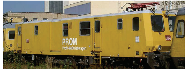
Fig. 5. PROM gauge limit measuring vehicle (marked as 712 002) [photo: Erik Rauner]
