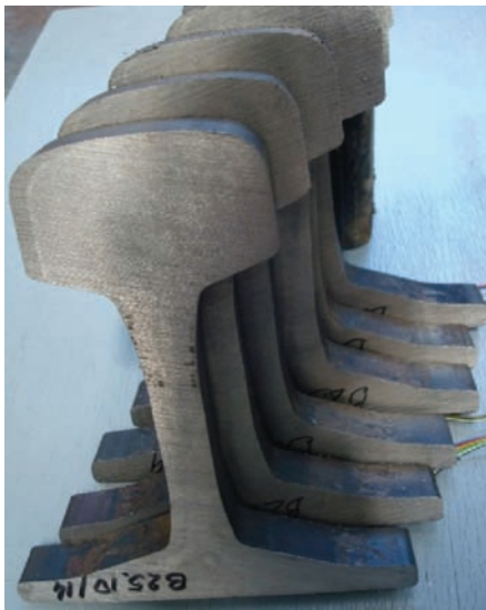
Fig. 4. Rails with stresses released [photo by the authors]
