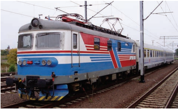
Fig. 5. Measuring train for pressure tests [photo by A. Zbieć]
