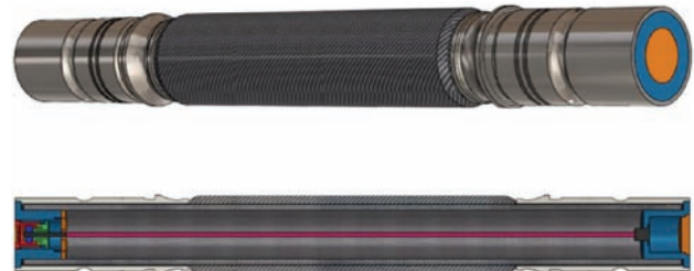
Fig. 3. Hybrid axle concept [6]
