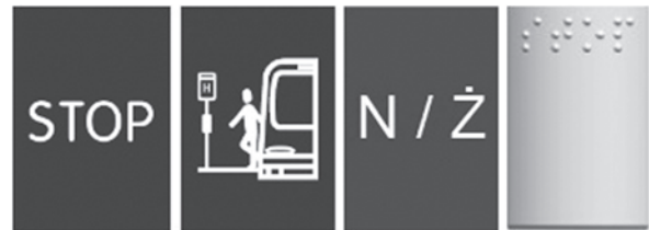
Fig. 3. Examples of visual and tactile information on a push button; own study based on [2]
