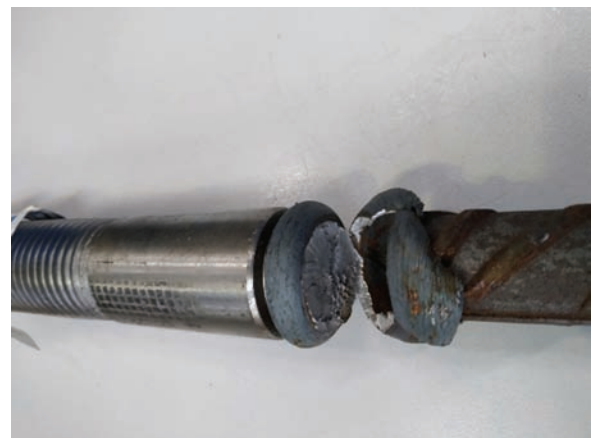
Fig. 10. Fracture of the weld in sample B23.4/21 [photo: M. Ostromęcka]
