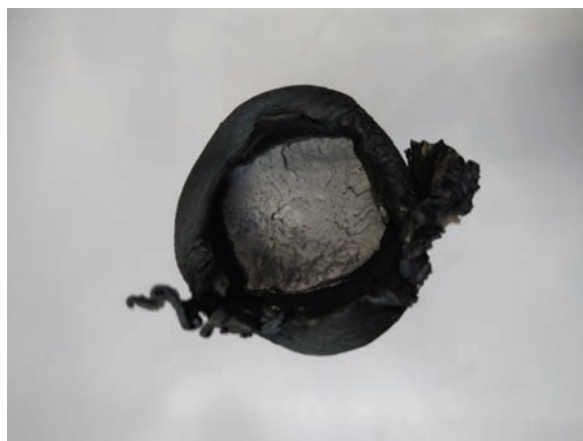
Fig. 8. Fracture of the weld in sample B22.5/21 [photo: M. Ostromęcka]
