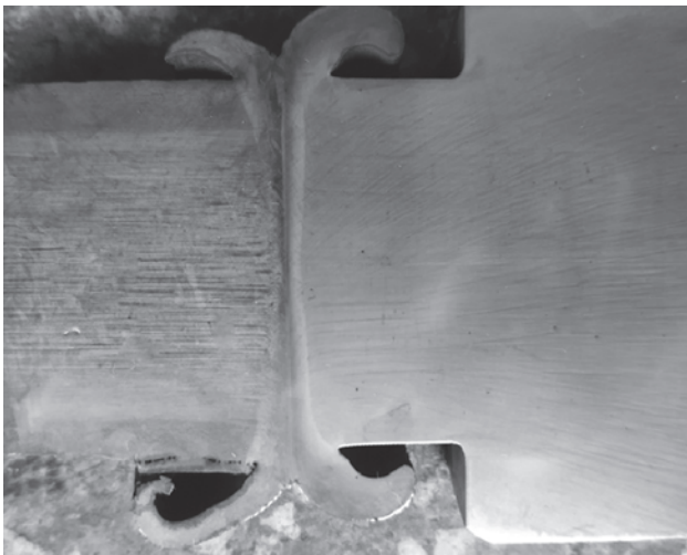
Fig. 3. Macrograph of a friction weld. Etching with Adler's reagent according to the withdrawn standard PN-61/H-04502 [4] [photo. M. Ostromęcka]
