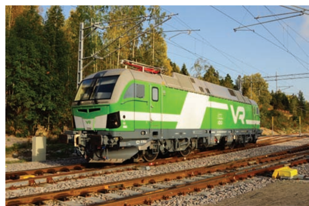
Fig. 23. Vectron VR 3306 locomotive (1524 mm, 25 kV 50 Hz) at Vanha Asema station, Finland (27 September 2017) [photo by P. Trippi]
