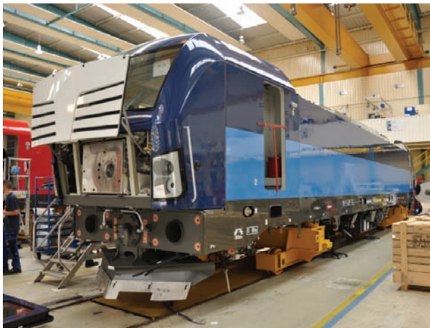
Fig. 9. Vectron locomotive for ČD during assembly at the Siemens Allach plant, Munich (27 June 2016) [photo by M. Graff]
