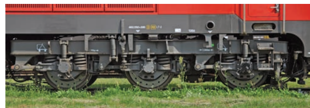
Fig. 14. The bogie of an LG-owned ER20 series (1,520 mm) locomotive [photo by M. Graff]
