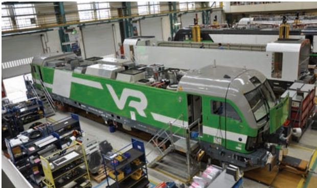
Fig. 25. Vectron locomotive for VR (1524 mm) during an assembly at the Siemens Allach plant, Munich (27 June 2016) [photo by M. Graff]
