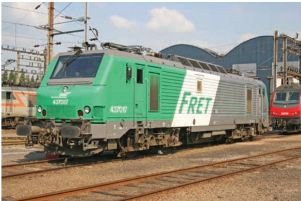
Fig. 1. Prima locomotive #437017 (1.5 kV; 15 kV 16.7 Hz; 25 kV 50 Hz) owned by SNCF Fret (Cargo); SNCF Lens-Méricourt locomotive depot, France (10 June 2005) [photo by L. Charlier]
