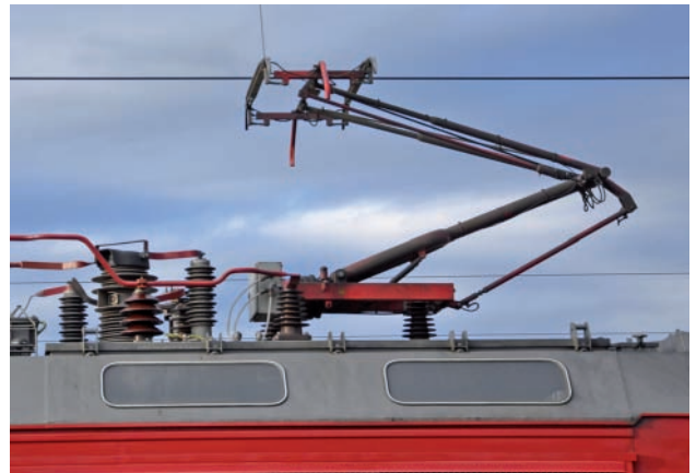
Fig. 42. A 361 series locomotive pantograph [photo by M. Graff]
