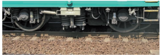
Fig. 33. A 151 series locomotive bogie [photo by M. Graff]
