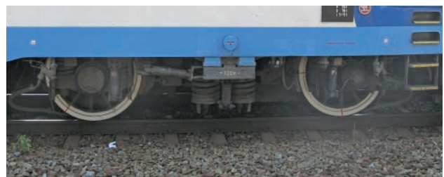
Fig. 37. A 350 series locomotive bogie [photo by M. Graff]
