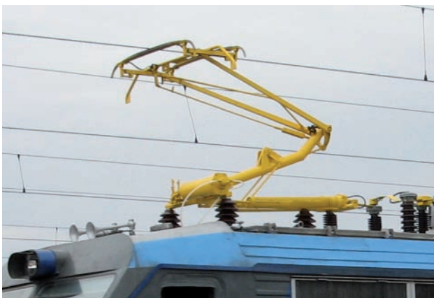
Fig. 45. A 350 series locomotive pantograph [photo by M. Graff]
