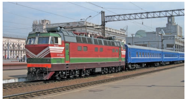
Fig. 5. CS4 T -603 (25 kV 50 Hz, 1,520 mm) with a long-distance train to Brest, Minsk (28 June 2006) [photo by M. Graff]
