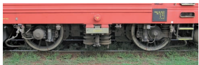
Fig. 36. A 263 series locomotive bogie [photo by M. Graff]
