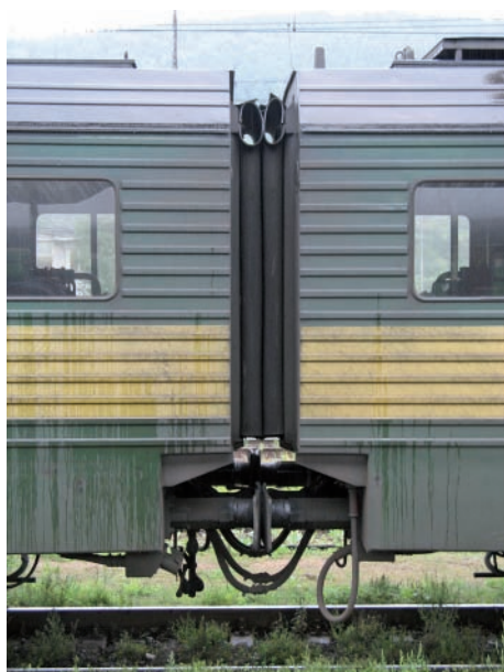
Fig. 16. The joint between the units of a 131 series locomotive [photo by M. Graff]
