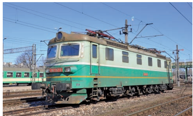
Fig. 2. 182 157 (3 kV DC, 1,435 mm) at the Białystok railway station (26 March 2011) [photo by M. Graff]
