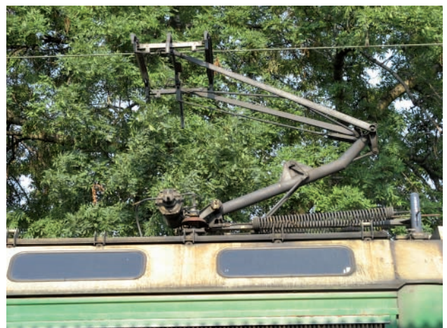
Fig. 43. A 163 series locomotive pantograph [photo by M. Graff]
