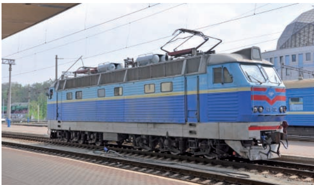
Fig. 4. CS4-132 (25 kV 50 Hz, 1,520 mm) at Kyiv station (1 May 2013) [photo by M. Graff]
