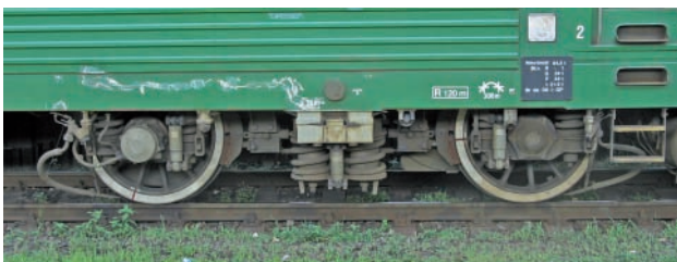
Fig. 31. A 163 series locomotive bogie [photo by M. Graff]
