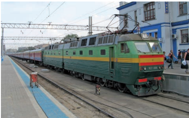
Fig. 3. CS7-088 (3 kV DC, 1,520 mm) with a long-distance train, Yaroslavsky Station, Moscow (29 June 2006) [photo by M. Graff]
