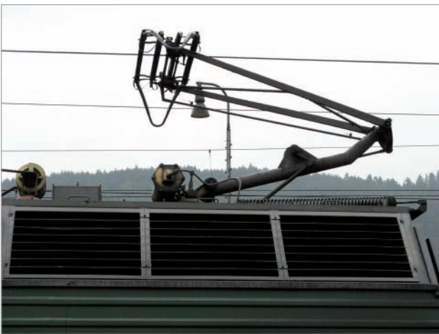
Fig. 39. A 131 series locomotive pantograph [photo by M. Graff]
