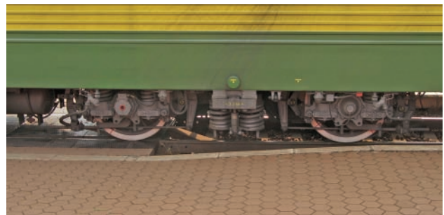
Fig. 34. A 131 series locomotive bogie [photo by M. Graff]
