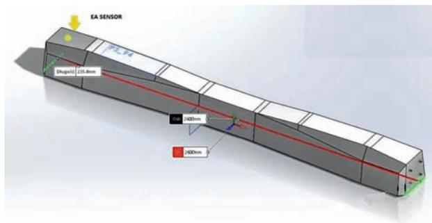
Fig. 4. The method of measuring the attenuation of the AE signal in the PS-94 prestressed concrete sleeper [the author's own compilation]
