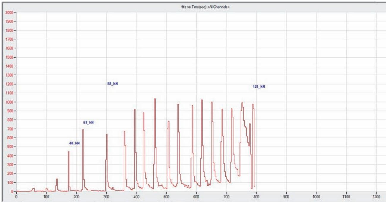
Fig. 19. Chart total energy [a] recorded on the basis of AE events until the destruction of the sleeper [the author's own compilation]
