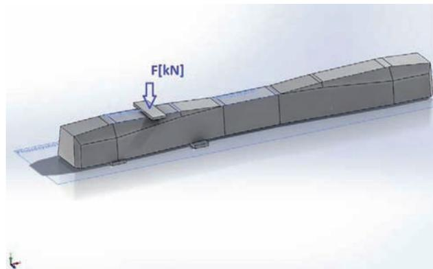
Fig. 10. Diagram of sleeper loads in the rail section [the author's own compilation]
