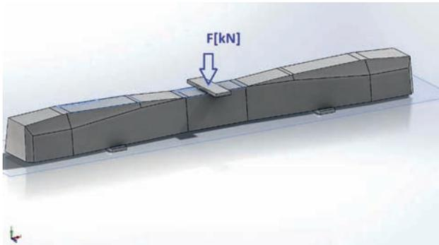
Fig. 11. Diagram of sleeper loads in the middle part in the normal position [the author's own compilation]
