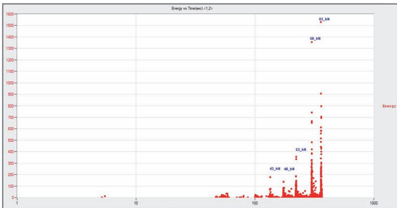
Fig. 17. The course of the load on the prestressed concrete sleeper \_1\_14 during the crack detection stage (time energy of events AE diagram) [the author's own compilation]
