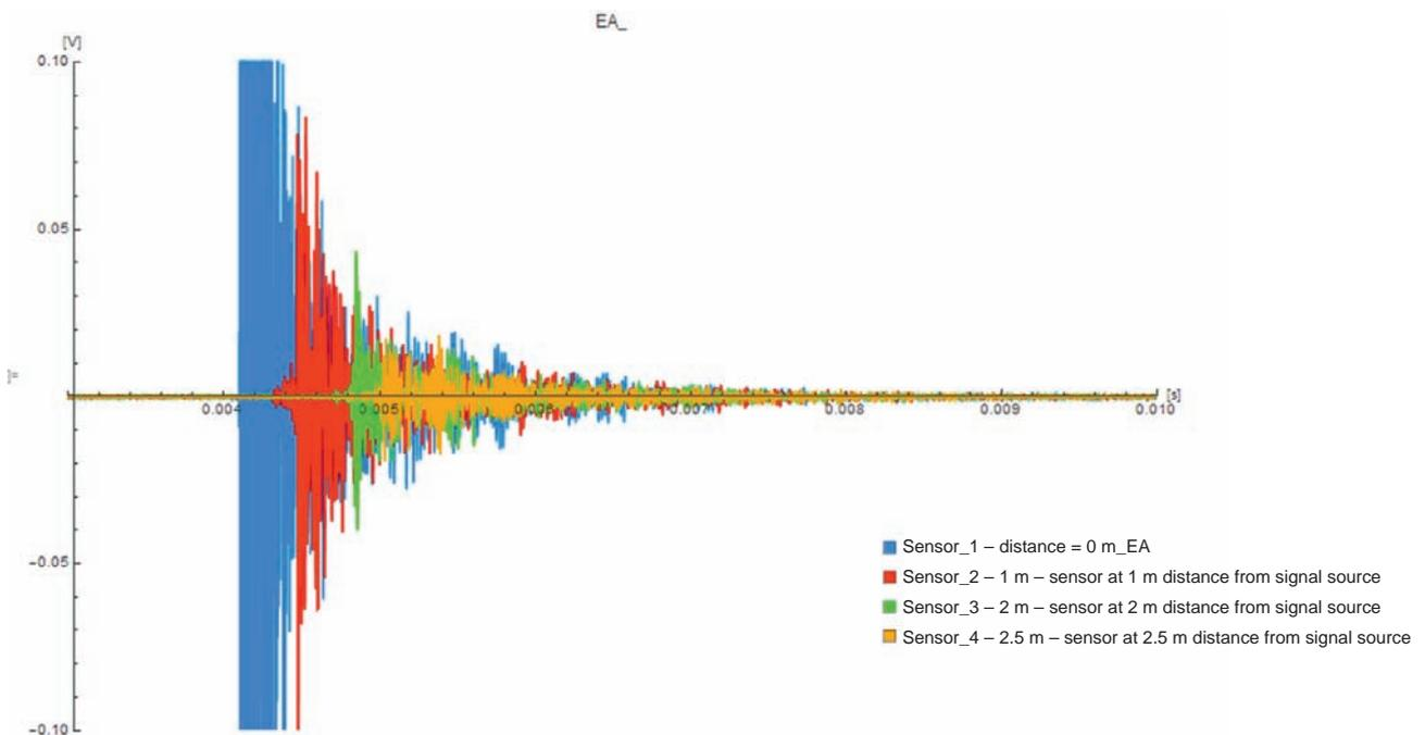
Fig. 8. Acoustic emission signals obtained on individual sensors at defined distances (according to Fig. 5) from the source of the AE event [the author’s own compilation]
