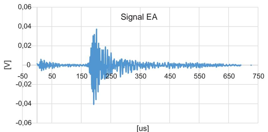
Fig. 3. An example of a real acoustic emission signal (AE) [the author's own compilation]
