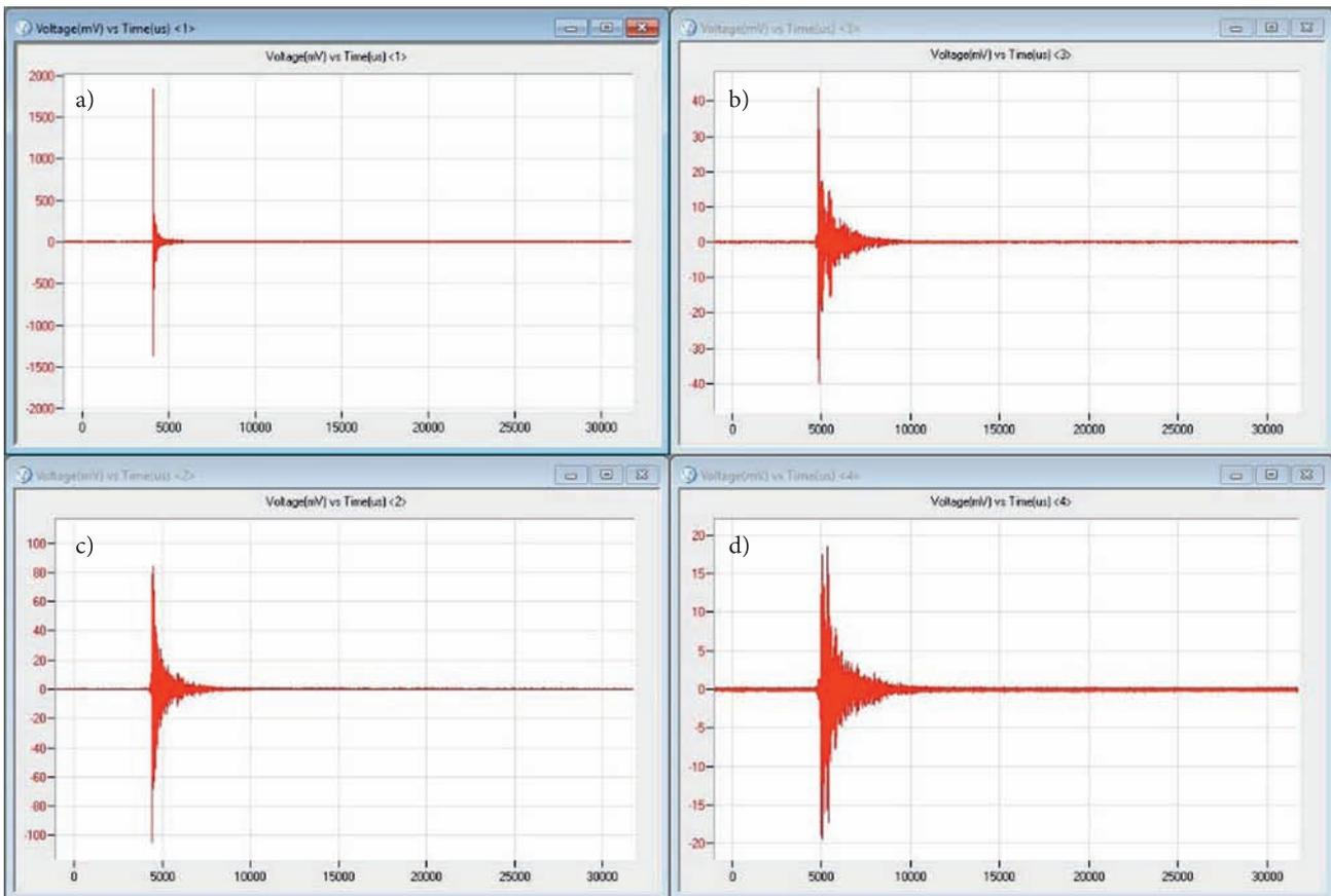
Fig. 7. Acoustic emission signal recorded on sensors of the same type located at different distances from the source (AE event site): a) 2.5 [m], b) 2 [m], c) 1 [m], d) 0.1 [m]; graph (Y-axis – voltage signal [V], X-axis – time [μs]; [the author’s own compilation]
