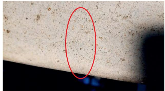
Fig. 14. The result of the visual inspection – finding the appearance of a crack during the loading of the sleeper [own elaboration]
