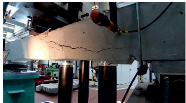
Fig. 15. Examination of a prestressed concrete sleeper on the LFV strength testing machine, load in the central part in an inverted position [photo D. Kowalczyk]
