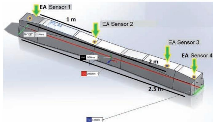
Fig. 6. The location of the sensors on the prestressed concrete sleeper during the determination of the attenuation of the AE (Hsu-Niesen) signals [the author’s own compilation]
