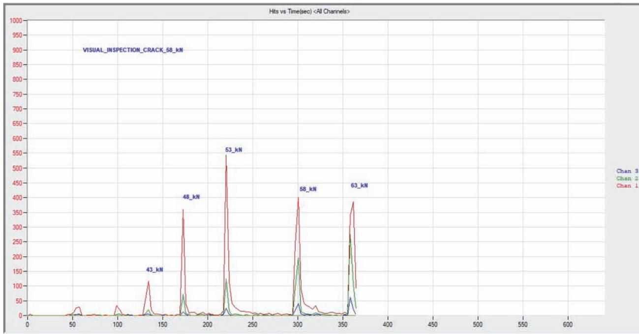
Fig. 18. The course of the load on the prestressed concrete sleeper marked as N\_1\_14 during the crack detection stage (number of AE events recorded on each sensor) [the author's own compilation]
