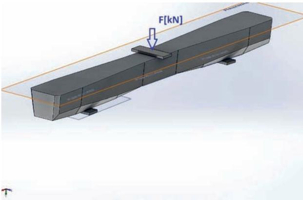
Fig. 12. Scheme of sleeper loads in the middle part in the inverted position [the author's own compilation]
