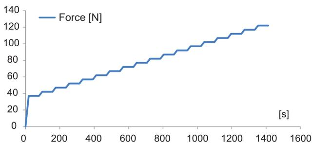
Fig. 13. Scheme of the sleeper load during the test in the middle part in the inverted position [the author's own compilation]
