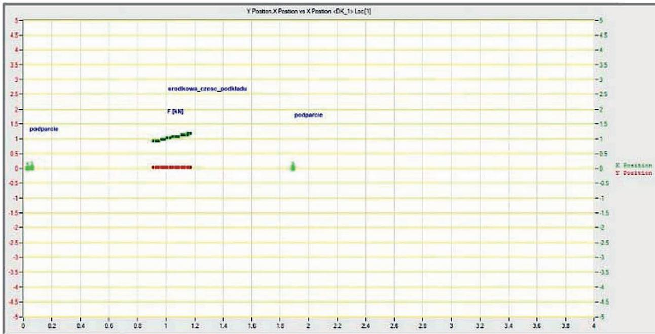
Fig. 16. An example of the occurrence of AE events in the sleeper in terms of loads for visual inspection of cracks (cracks) on the sleeper surface (about 63 kN – load in the middle part of the sleeper) [the author's own compilation]
