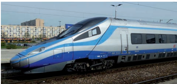
Fig. 6. The nose of the ED250 (Pendolino) electric multiple unit [Photo by A. Zbieć]
