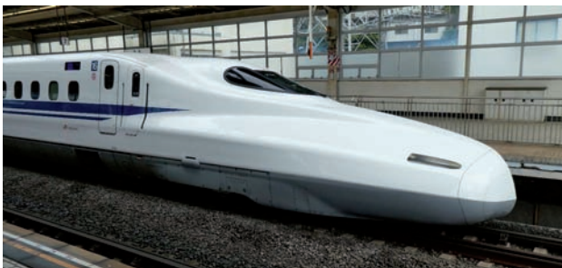
Fig. 5. The long nose of the Japanese Shinkansen N700-series high-speed vehicle [Photo by A. Zbieć]
