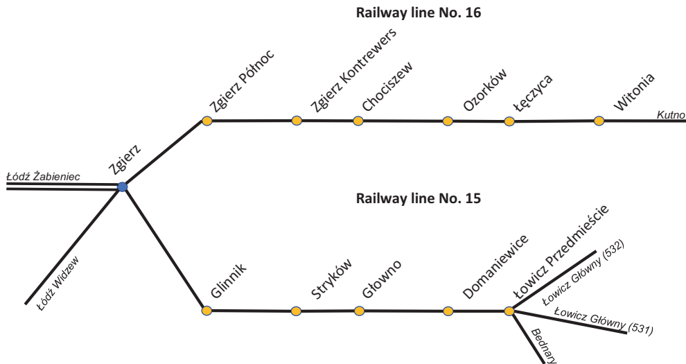
Fig. 16. Layout of railway lines covered by the study; orange dots indicate stations whose sectioning diagrams are included in figures 17–27 [own work]
