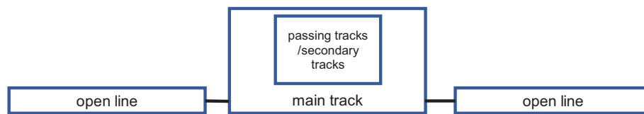
Fig. 11. Supply of station tracks (groups of tracks) from the main track contact line [own work]
