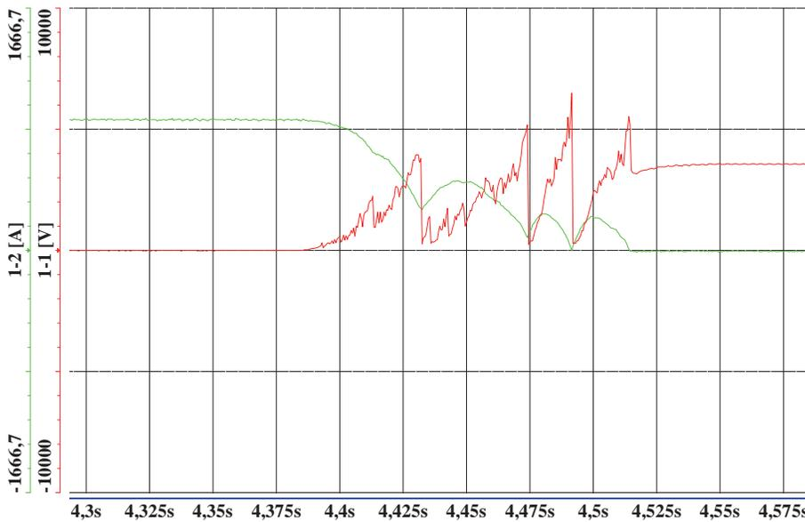
Fig. 10. Multiple arcing events during current breaking by the contactor due to poor condition of the arc box
