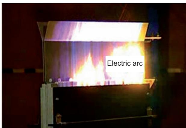
Fig. 2. Arc box and electrical arc formed during the disconnection of direct current by a high speed circuit breaker [13]
