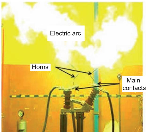
Fig. 1. Electrical arc formed during the disconnection of direct current by a switch disconnecter [13]
