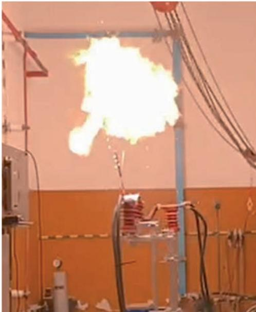
Fig. 12. Plasma ball after current breaking by the switch disconnecter [photo taken by M. Marszałek]
