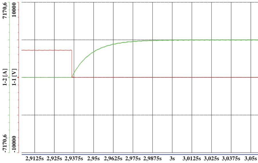
Fig. 14. Waveform of correctly switched-on current by the switch disconnector
