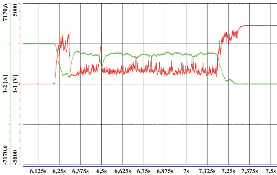
Fig. 16. Arc ignition between the main contacts of the switch disconnector during current breaking
