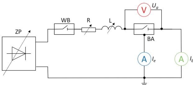
Fig. 3. Schematic of the measurement system for electrical endurance testing (description in the text) [own work]
