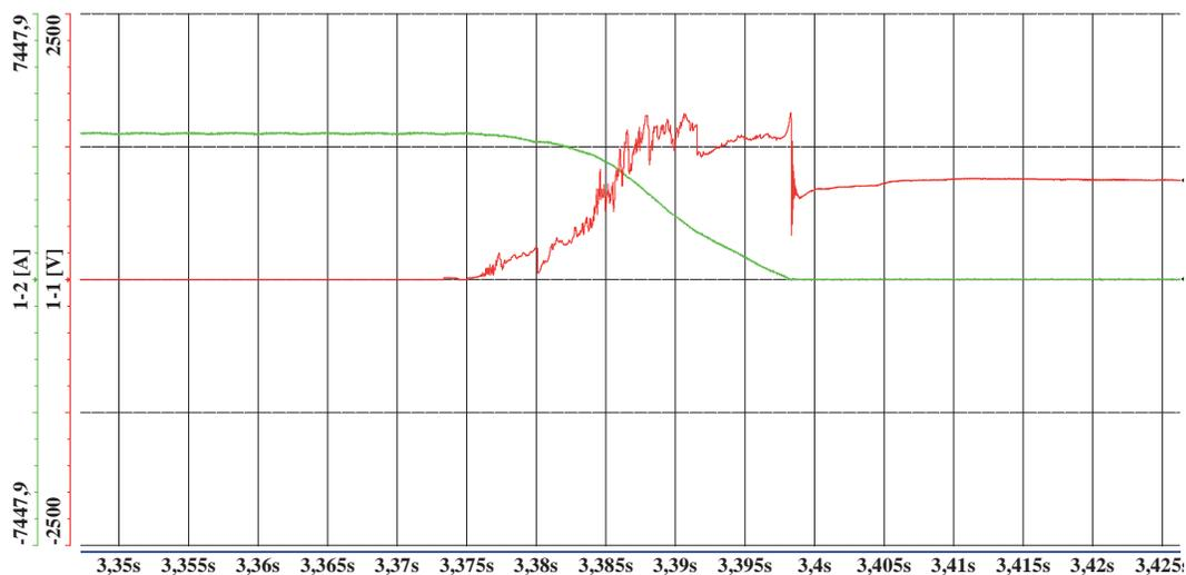
Fig. 4. The waveforms of the switched current and arc voltage when properly switched off by a high speed circuit breaker<sup>2</sup>
