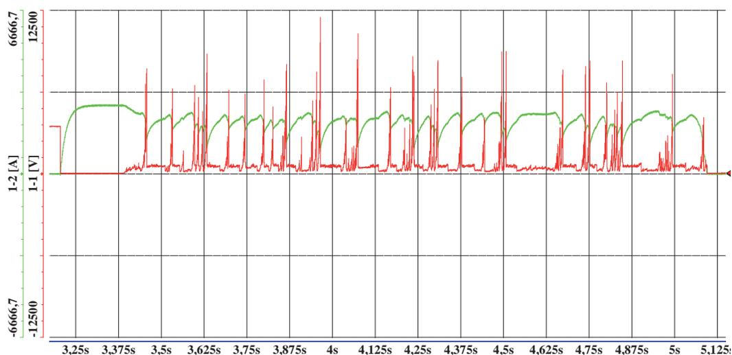
Fig. 5. Waveforms of the switched-off current and arc voltage during multiple breakdowns of the inter-contact gap of the high speed circuit breaker due to poor technical condition of the arc box
