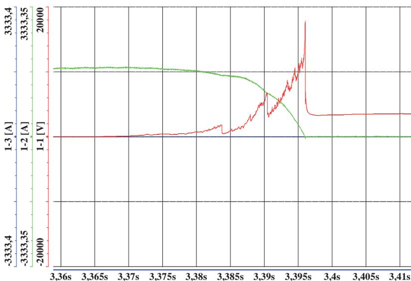
Fig. 7. Waveforms of switched-off current and arc voltage reaching excessively high values
