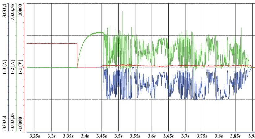
Fig. 6. Waveforms of circuit currents and arc voltage during ground fault
