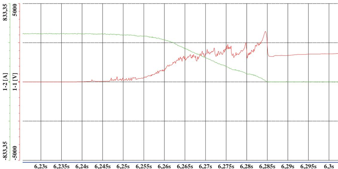
Fig. 9. Typical voltage and current waveform during current breaking by a contactor
