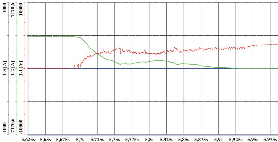
Fig. 13. Voltage waveform across the switch disconnecter and switched-off current
