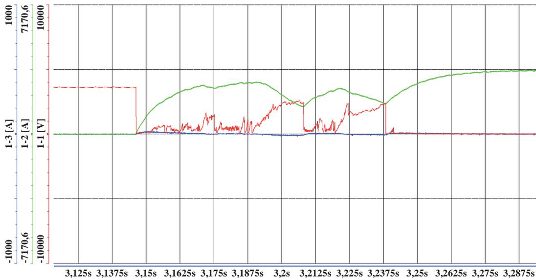
Fig. 15. Arc ignition during current switching by the switch disconnector due to insufficient contact condition
