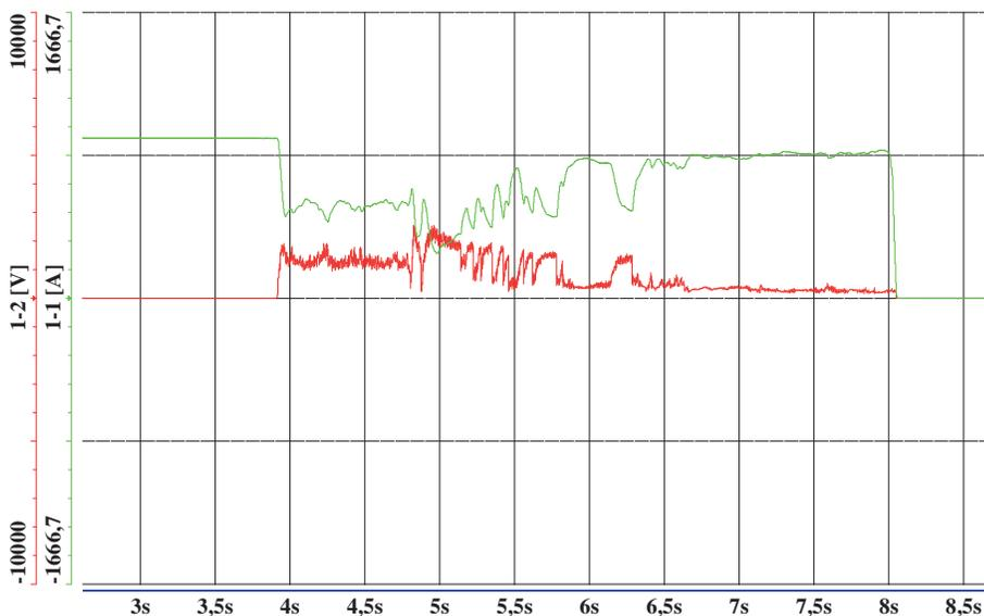
Fig. 11. Failure to break the current due to too low arc voltage
