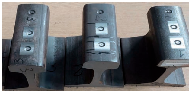
Fig. 4. Sections of the three rail grades used in the tests [photo by I. Mikłaszewicz]
