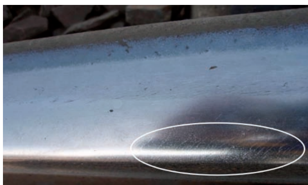
Fig. 1. Rail head checks at their initial stage [photo by I. Mikłaszewicz]
