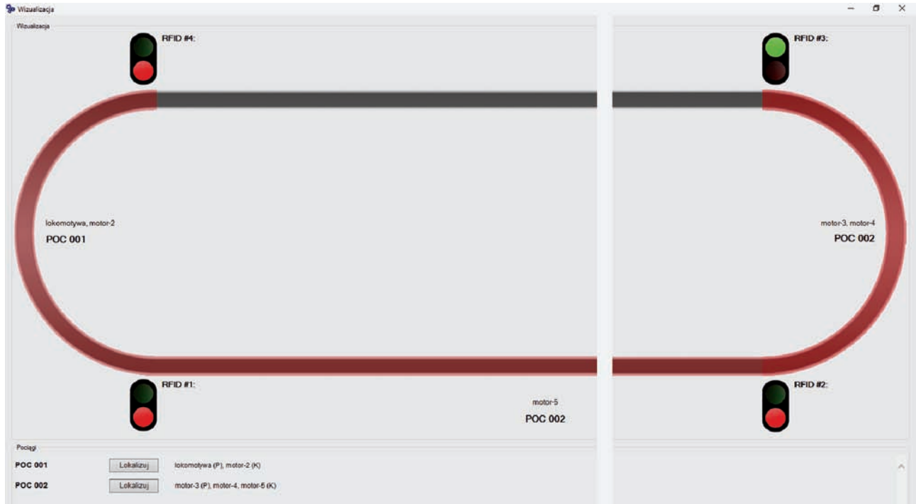
Fig. 12. Three experimental track sections, occupied by trains POC-001 and POC-002 [J. Moczarski's resources]
