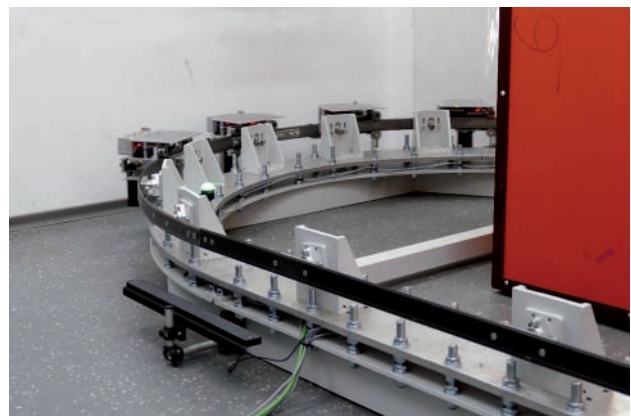
Fig. 10. The next section is empty – a signal to proceed is given (green light) [photo by J. Moczarski]
