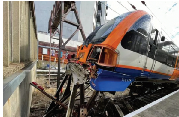
Fig. 21. Train derailment (12 October 2021) in London at Enfield Town Station; collision with a fixed buffer stop, view from the platform side [9]
