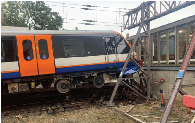
Fig. 20. Train derailment (12 October 2021) in London at Enfield Town Station – collision with a fixed buffer stop [9]
