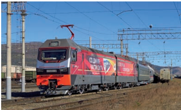
Fig. 5. 2ES7-001 (25 kV 50 Hz) during trials at the East Siberian Railway of RZD (10/10/2016) [photo: Ural Locomotives]
